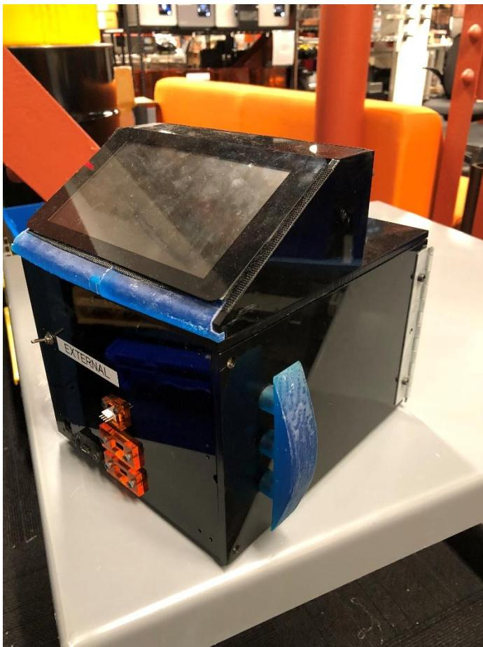
Purpose: Test lasers for optical power and surfaces for attenuation
